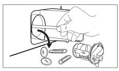
9. Check carefully whether the pump impeller rotates (it rotates jerkily). If it doesn't rotate, please contact your Service Centre.
